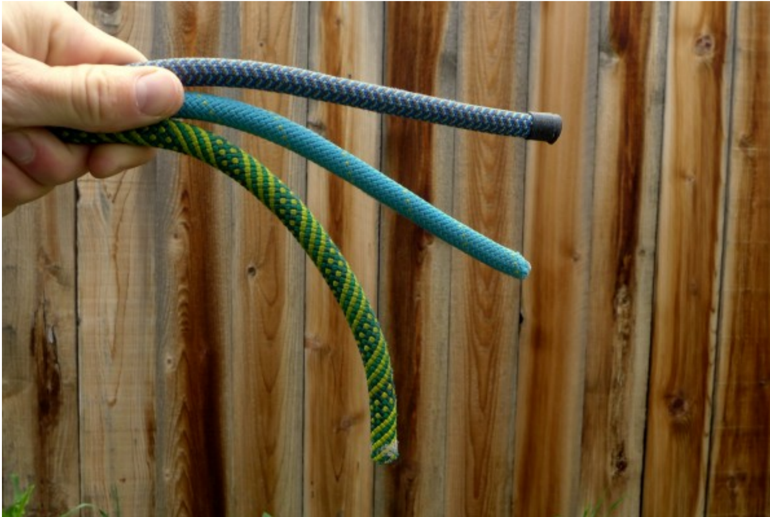
Some ropes that initially handled well became stiff after heavy use. Here is a comparison between three different workhorse ropes at the end of testing, from top to bottom: New England Alex Honnold Glider, Mammut Sensor, Sterling Marathon Pro. The Marathon Pro felt the nicest to handle when actually climbing.
