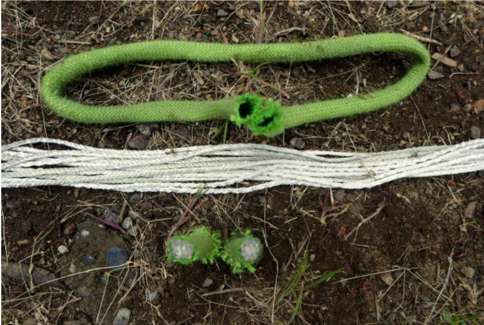
String Theory: A kernmantle rope has two parts, the hollow tube of the sheath (green) and the twisted fibers of the core (white). At the bottom you can see how they are arranged in cross section.
